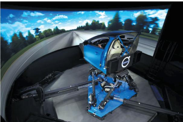
Fig. 5. Volvo Dynamic Driving Simulator [6]
