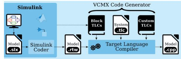
Fig. 2. Code generation process of Simulink [2]
