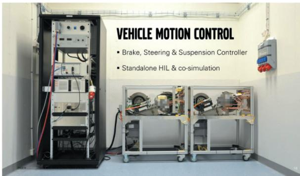
*Fig. 3. This vehicle motion control HIL system tests braking, steering, and suspension controllers. The system can act as a stand-alone HIL test setup or be run in co-simulation with the Dynamic Driving Simulator [6]*
