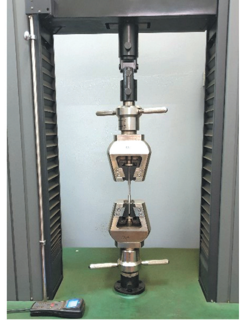
Fig. 6. Spectrometer examination of the chemical composition of structural components (a); tensile machine for tearing metal samples (b)
