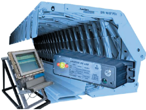
Fig. 6. The active pressure maintenance system from Elsta [22]
