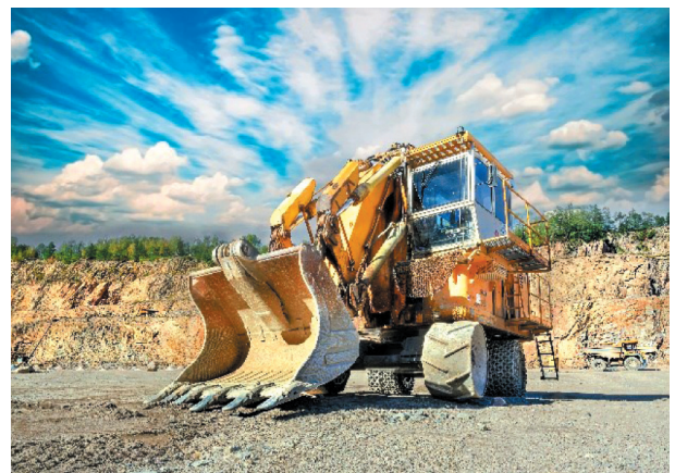
Fig. 11. Bola LB-600 single-bucket hydraulic front shovel
