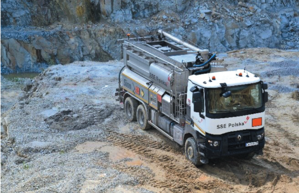
Fig. 7. Blasting rig produced by SSE [6]
