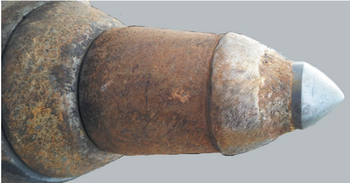
Fig. 4. Incorrect sizing of the sintered carbide insert to the hardness of the body and mining conditions
