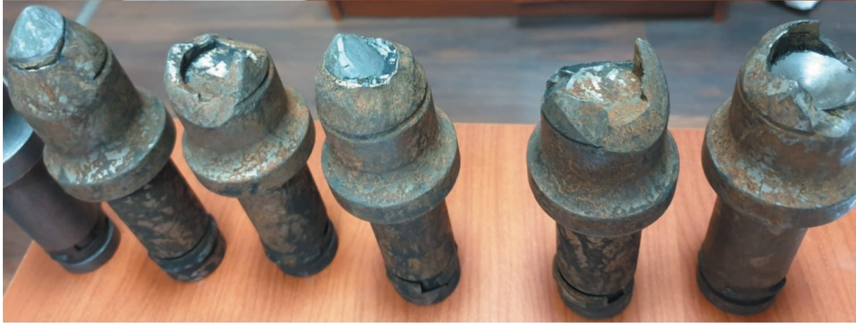
Fig. 2. Bits after one day of working from an unknown competitor
