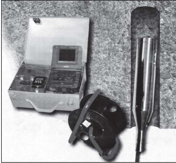
Fig. 1. Introsopic camera to examine rock structure penetrated by drilling operations
